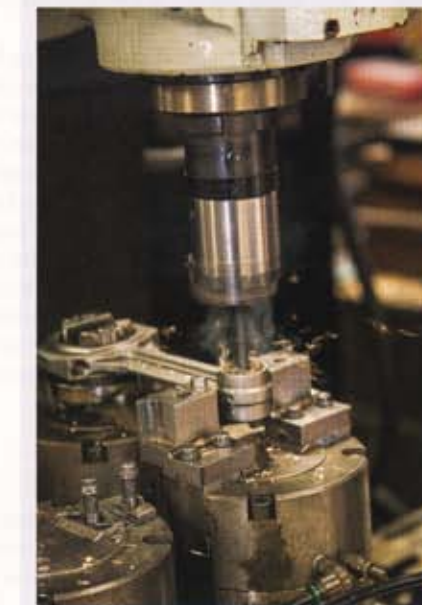
Pauter rods are made from billet block at the family-run Pauter shop in San Diego.
