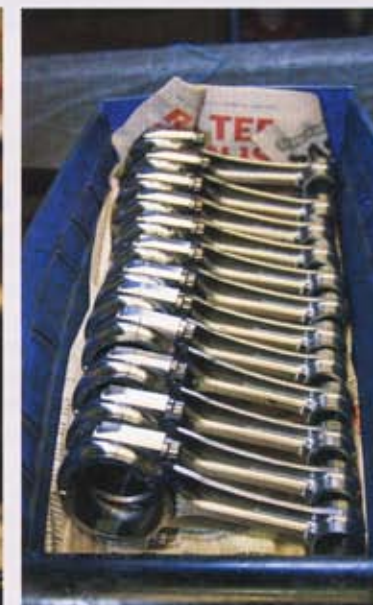
Pauter rods are made from billet block at the family-run Pauter shop in San Diego.
