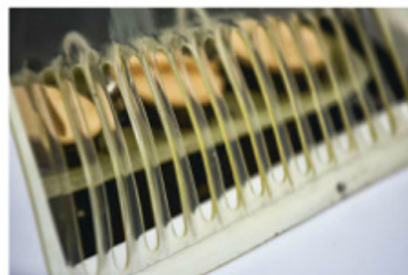
Jürgen Barth drove 907-003 at the Daytona Classic. As it did at Le Mans in 1967, 907-003 runs a flat six, which breathes through louvers cut into the clear rear engine cover.
