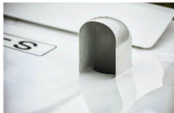
Porsche engineers designed the air inlets to avoid aerodynamic disturbances—both up front for the front-mounted oil cooler and at the rear, where scoops (left) help to keep transmission temperatures in check. The rear deck was also fitted with an adjustable rear spoiler (left) to improve high-speed stability.
