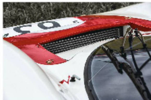
The wind-tunnel-honed 907-003 streamliner was sleek, but it was aerodynamically unstable in initial tests. The car incorporated a Plexiglas cover over the engine, a tall windscreen, doors with flush windows, and an adjustable rear spoiler.
